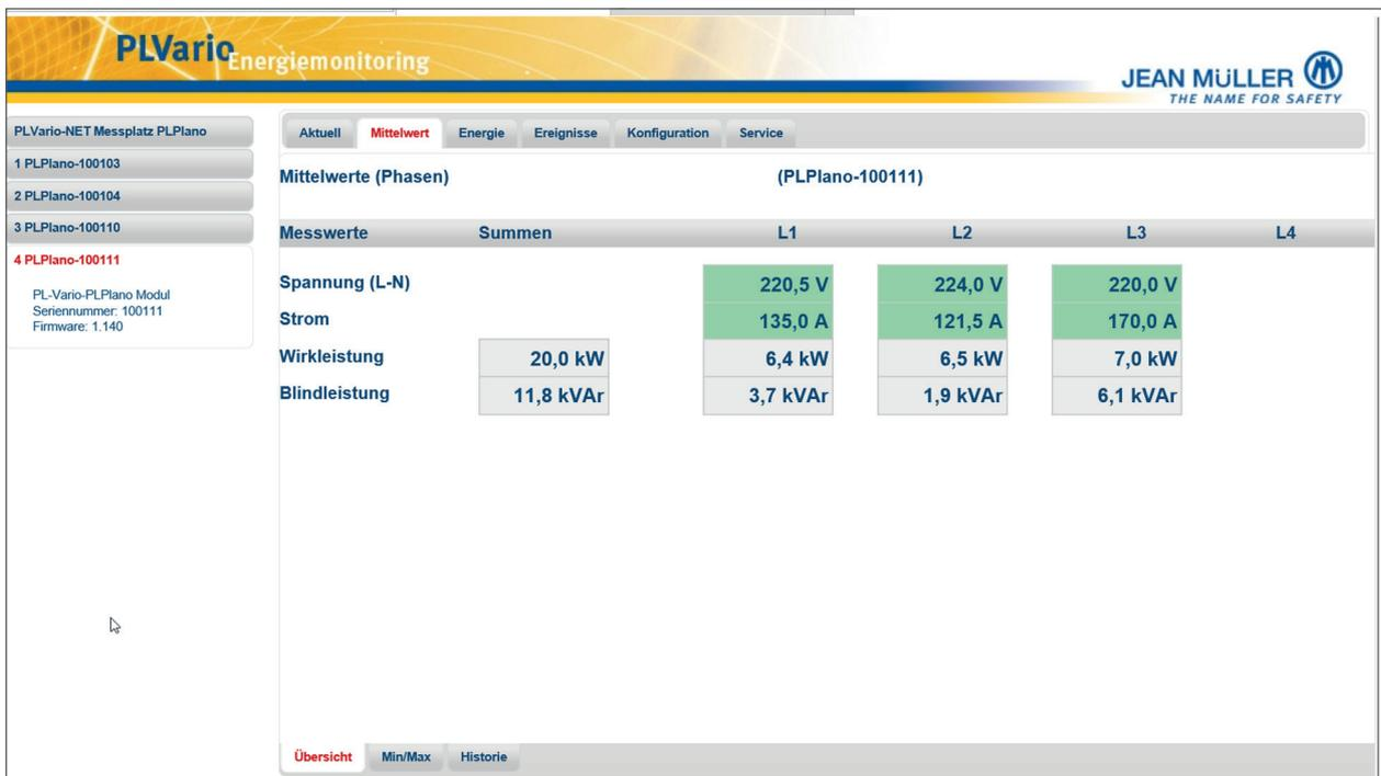
The screenshot shows the 'Mittelwert' (Average) menu for phase data. The interface includes a navigation bar with 'Aktuell', 'Mittelwert', 'Energie', 'Ereignisse', 'Konfiguration', and 'Service'. The main content area displays a table of average values for four phases (L1, L2, L3, L4) across four categories: Spannung (L-N), Strom, Wirkleistung, and Blindleistung. The 'Summen' (Totals) column is also visible.
